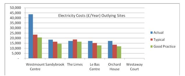
The graph above indicates that the Westmount Centre issues highlighted during the survey, such as the problems lighting and its control installation and domestic water services booster pumps are likely to be having a very significant impact on the cost of running this building; and further analysis of the half hourly data will help to identify this. There is also scope to reduce consumption on the other sites, albeit much reduced.
